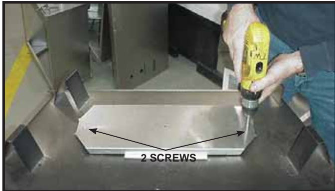
Figure 9.1 For top vent, remove the two screws holding the top heat shield in place. For rear vent, see Section 9.B.
